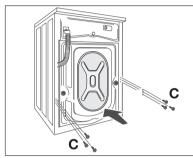
**7.** Open the porthole and remove the polystyrene block fitted with the adhesive tape on the door seal.
